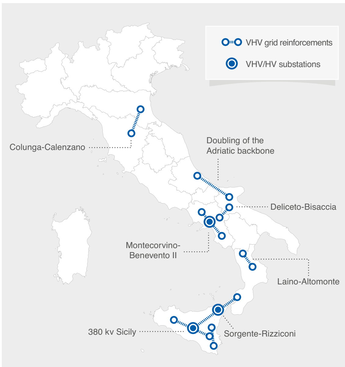
Figure 2 - Main action on the 380 kV grid aimed at greater production from RES.
